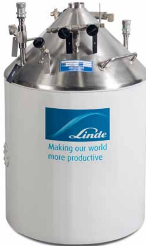
**Application area** The cryogenic adsorber is recommended for clean-up of the helium gas in a liquefier or refrigerator system which has been opened and exposed to the atmosphere. It is especially effective for removal of air and moisture and saves time compared with the usual procedure of pumping and purging.
