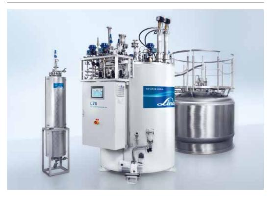
The newly developed, fully automatic computer controlled L-Series offers a wide range of liquefaction and refrigeration capacities, depending on liquid nitrogen ( $LN_2$ ) pre-cooling and on the chosen size of compressor. All standard coldboxes are equipped with a  $LN_2$  pre-cooling facility, which allows a significant increase in capacity. The L70/LR70 therefore provides a high degree of flexibility to meet your requirements today and in the future.
